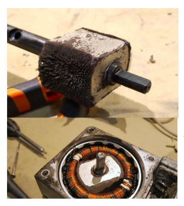
The second most common problem is that magnetic assembly internally breaks up and this makes the flap stick and there is a lot of friction over the whole flap movement.
