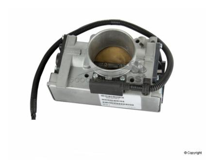
The throttle bodies can have one of 4 problems. Most common is the rotary sensors fail causing errors (usually P225). These can be replaced with contactless sensors which do not suffer from the physical wear that the originals ones do, and will most likely last a lot longer without trouble.
